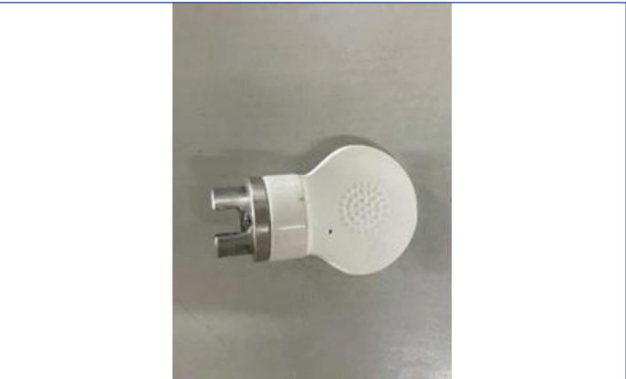
[Table/Fig-7]: Upper limb pronation supination component of Rymo-Mobi-L machine.
